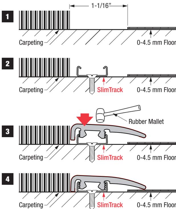
*If the flooring manufacturer suggests/permits the use of underlayments, you may need to shim the track to accommodate the increase in overall thickness*
