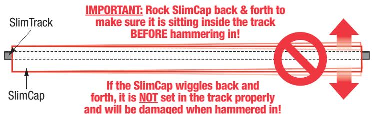
**Step 4:** Next, go up and down the molding several times, tapping the SlimTrim all the way into the track. You can use a little more force once you are sure it is properly engaged in the track.
