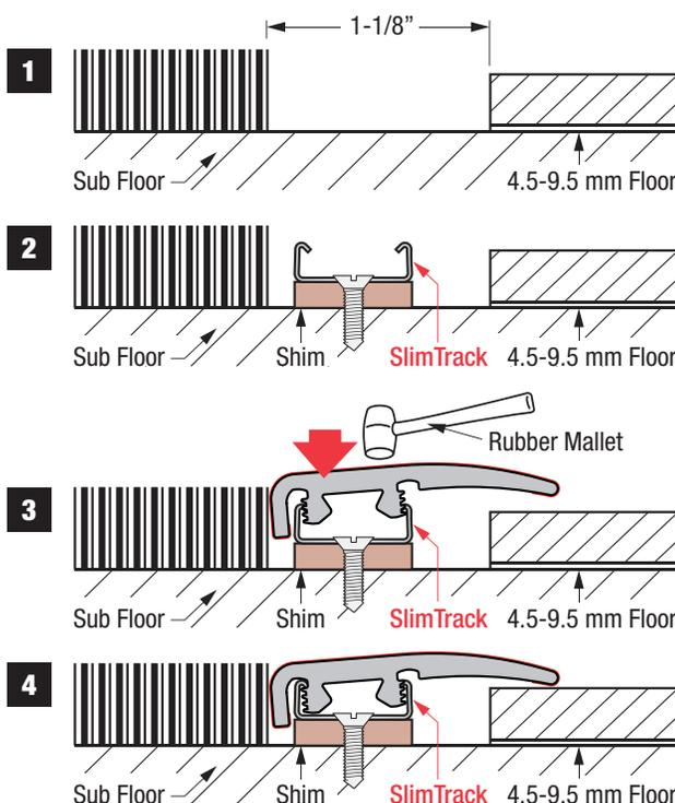
**Step 1:** Install the flooring planks including the underlayment by leaving a 1-1/16" inch (27mm) gap for the installation of the SlimCap molding.
