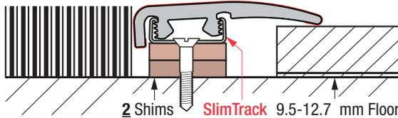
**Step 1:** Install the flooring planks including the underlayment by leaving a 1-1/16" inch (27mm) gap for the installation of the SlimCap molding.
